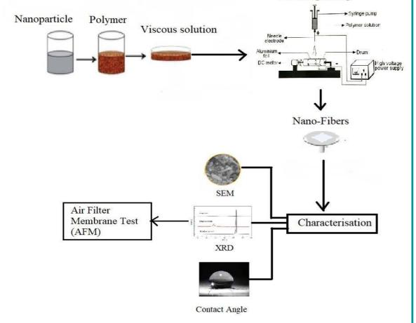
This instrument produce nanofibers later it is characterized by scanning electron microscope (SEM) where the electron beam is used to scan the surface of a sample to create images with an electron microscope and it can only produce two dimensional views. ImageJ was used to calculate the diameter of the fiber.
